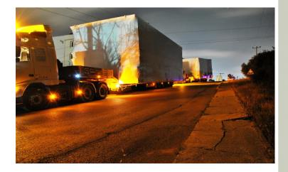
Leadingengineeringcompany of France has selectedCanlogisticfortheroadtransportation of Cooler&Granulatorsections, total 9 units, each 17 meterslong, 6 meterswidhtand 7,5 metersheight (54 tons) from Gebze factorytoEfesan Port in Dilovası.
